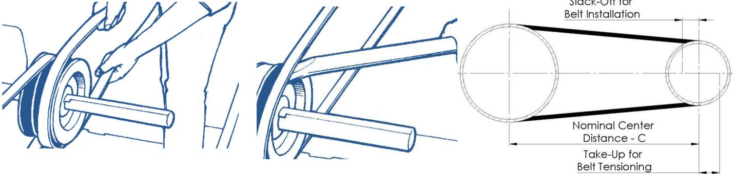
6. The nominal center distance should be determined from a standard pitch length and designed so that the centers can be moved closer together and farther apart to allow for installation and tensioning. The following tables are minimum allowances which allow for manufacturing tolerances as well as stretch and wear of belt. If the drive was designed following the guidelines below, there should be no problem installing or tensioning a belt of the correct length on the drive.
