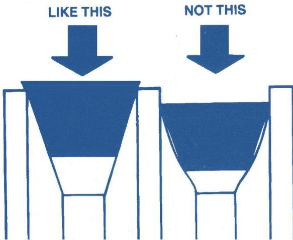
2. Inspect pulleys for wear. Worn pulleys greatly reduce belt life. Extreme wear can lead to belts bottoming in grooves. The result is slippage and excessive heat buildup. Use a pulley groove gauge to check for wear. V-belts should ride at least flush with the top of the pulley and may ride out up to 0.2". Check for burrs, nicks, gouges and severe scratches as these will drastically reduce belt life. Replace if necessary.
