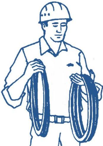
4. Ensure all belts are the same. Do not mix belt brands. Do not mix belt constructions. (Such as raw edge, cogged, wrapped, single and banded) Do not mix new and used belts. The new belt or belts will carry the entire load. Do not mix used belts from different drives. Any mixed belts will cause the load to be carried unevenly, causing the belt carrying the majority of the load to fail rapidly, followed by the remaining belts.
