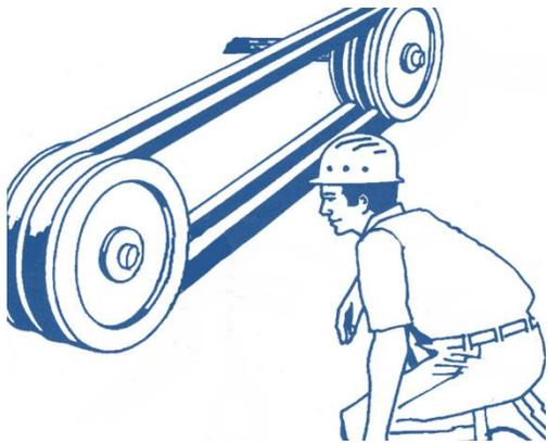
Properly installed belts generally do not require much maintenance. V-Belt drives are recognized as extremely reliable, trouble free and efficient. The main ingredient of good maintenance of a belt drive is to look and listen. Any of the following can be detrimental to belt life but if corrections are made and the belts have not been damaged, the drive will continue to perform well.
