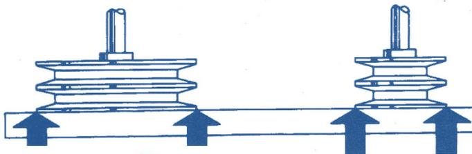
Use a straightedge to check drive alignment. All four points of the straightedge should contact the pulley. Use the straightedge in different positions to check for all kinds of misalignment. In multi-belt drives, misalignment can cause belts that are actually all the same length to appear different lengths. Extreme misalignment can cause rollover and severe belt wear.
