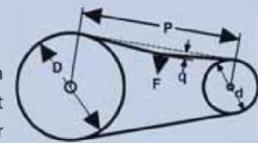
to deflect the belt 1/64" for each 1" of belt span, q. So, for a 32" span, the deflection amount would be 32/64" or 1/2".
